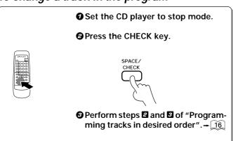
Press the CHECK key repeatedly until the track No, to be changed is displayed.
